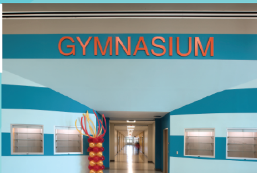
12" HIGH PAINTED ALUMINUM WITH 1/2" PROJECTION
