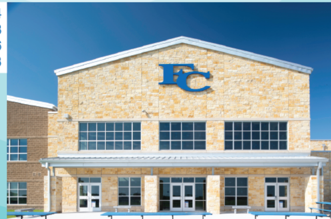
8" HIGH FABRICATED STAINLESS STEEL, PAINTED FACE LOGO, BACK LIT (HALO)
